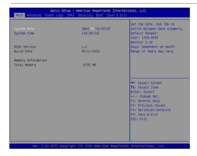
The Main BIOS setup screen has two main frames. The left frame displays all the options that can be configured. Grayed-out options cannot be configured; options in blue can. The right frame displays the key legend. Above the key legend is an area reserved for a text message. When an option is selected in the left frame, it is highlighted in white. Often a text message will accompany it.
