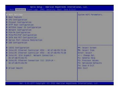
Warning: Take caution when changing the Advanced settings. An incorrect value, a very high DRAM frequency, or an incorrect DRAM timing setting may make the system unstable. When this occurs, revert to default manufacturer settings.
