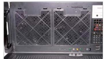
The washable fan filter can be easily taken off to make an easier maintenance.
