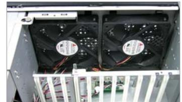
Equipped with dual 12cm ball bearing fans, AREMO-4196 provides the best ventilation up to 208CFM to expire heat from the system.
