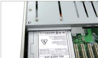
Flexible design to install power supply, the bracket can be adapt to PS/2 type or mini-redundant power supply.
