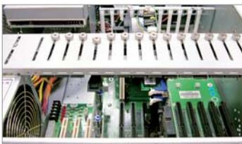
AREMO-4196 adopts the newly designed card retainer to hold both the PCI and ISA type add-on-cards more tightly.
