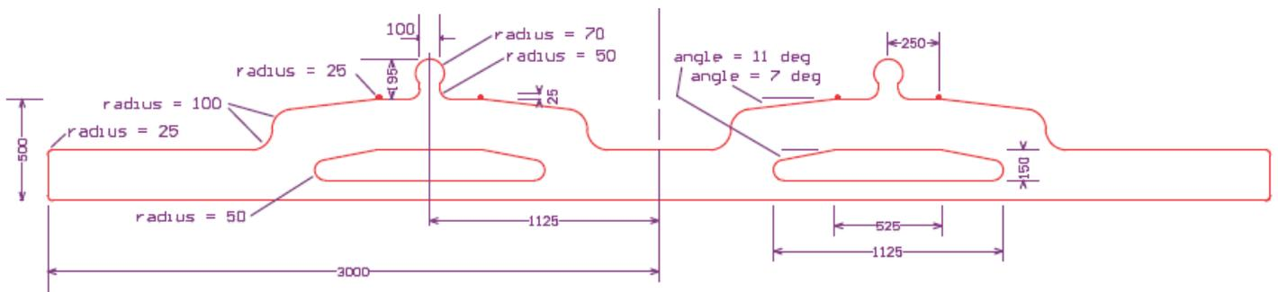
**Figure 3: Cross Section of Shock Mount Pad**
