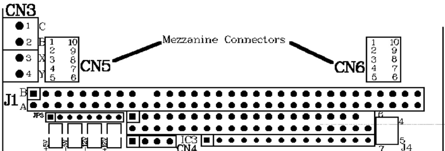
in the range of 6.5 to 20VDC through the Battery Power Connector CN3. Two external signals can be connected to the battery terminal block for use by add-on modules plugged into the mezzanine header connectors. Connect to the HE104 Battery Terminal Block as follows:
