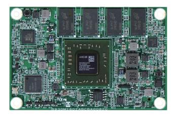
MEDM-MBA0 is designed with AMD Quad core G-Series SoC solution and Mini Com express type 10 form factor which is specifically designed for customers who need high-level processing and graphics performance with low power consumption in a long product life solution.
