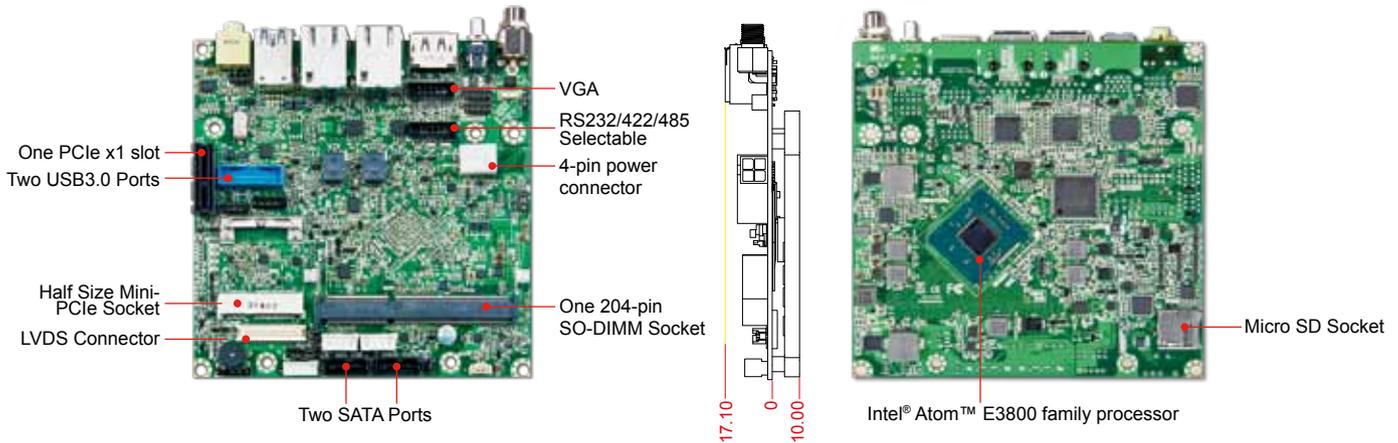
NANO-6060, built with Intel® Atom™ processor E3800 family that not only outputs under 10W for fanless applications, but also supports a wide industrial temperature from -40°C to 85°C, delivers superior up to quad-core processing power and high capability. Portwell has taken advantage of such technology to furnish a series of products that can meet multiple industrial requirements such as fanless, cost-effective of CPU performance, and compact systems.
