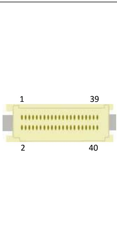
**CN17: Front panel pin header**
