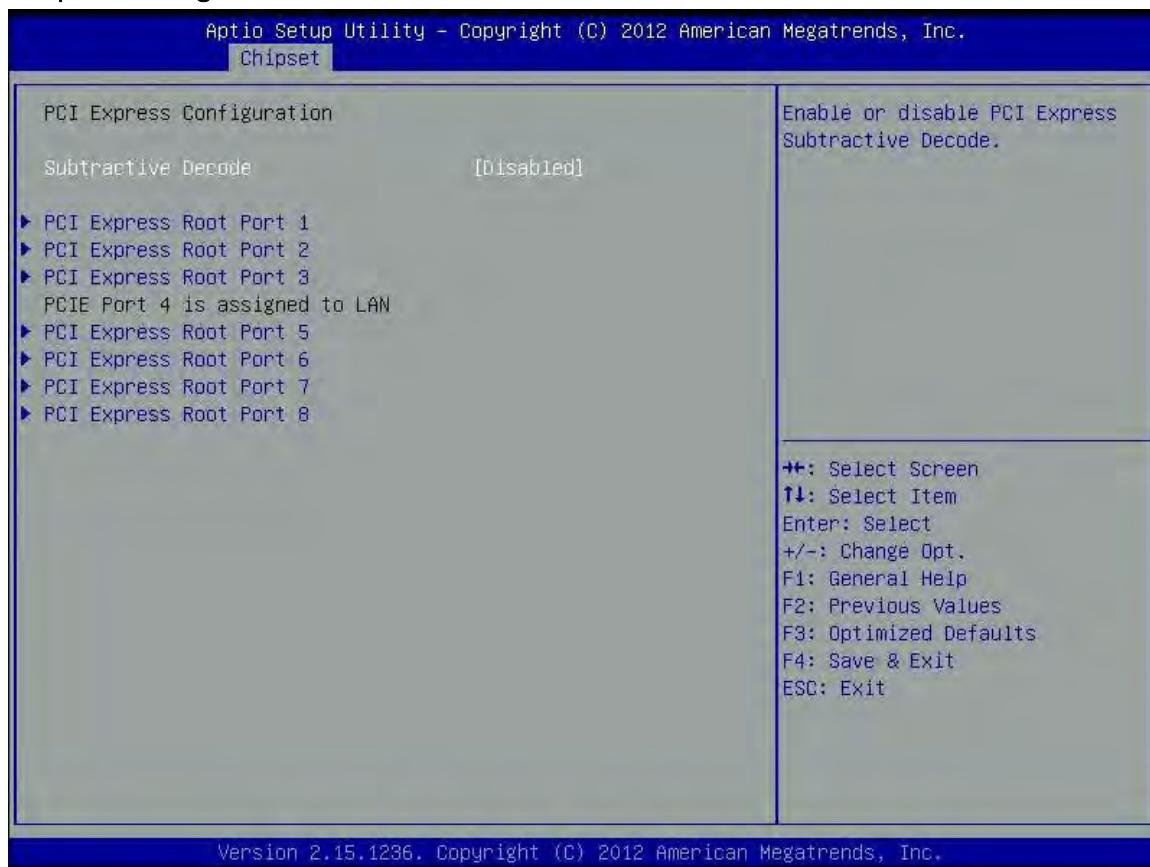
**Subtractive Decode:** Enable or disable PCI Express Subtractive Decode.
