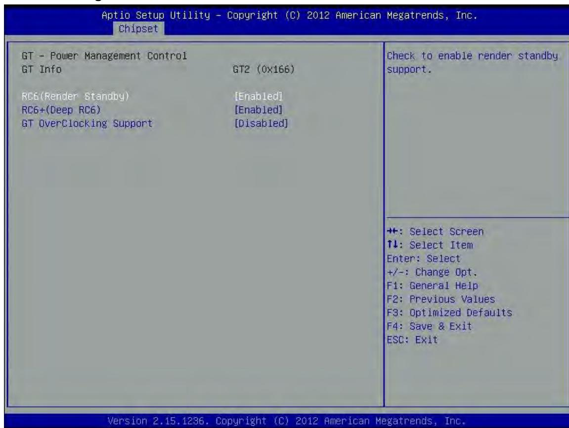
**RC6 (render standby):** check to enable render standby support.
