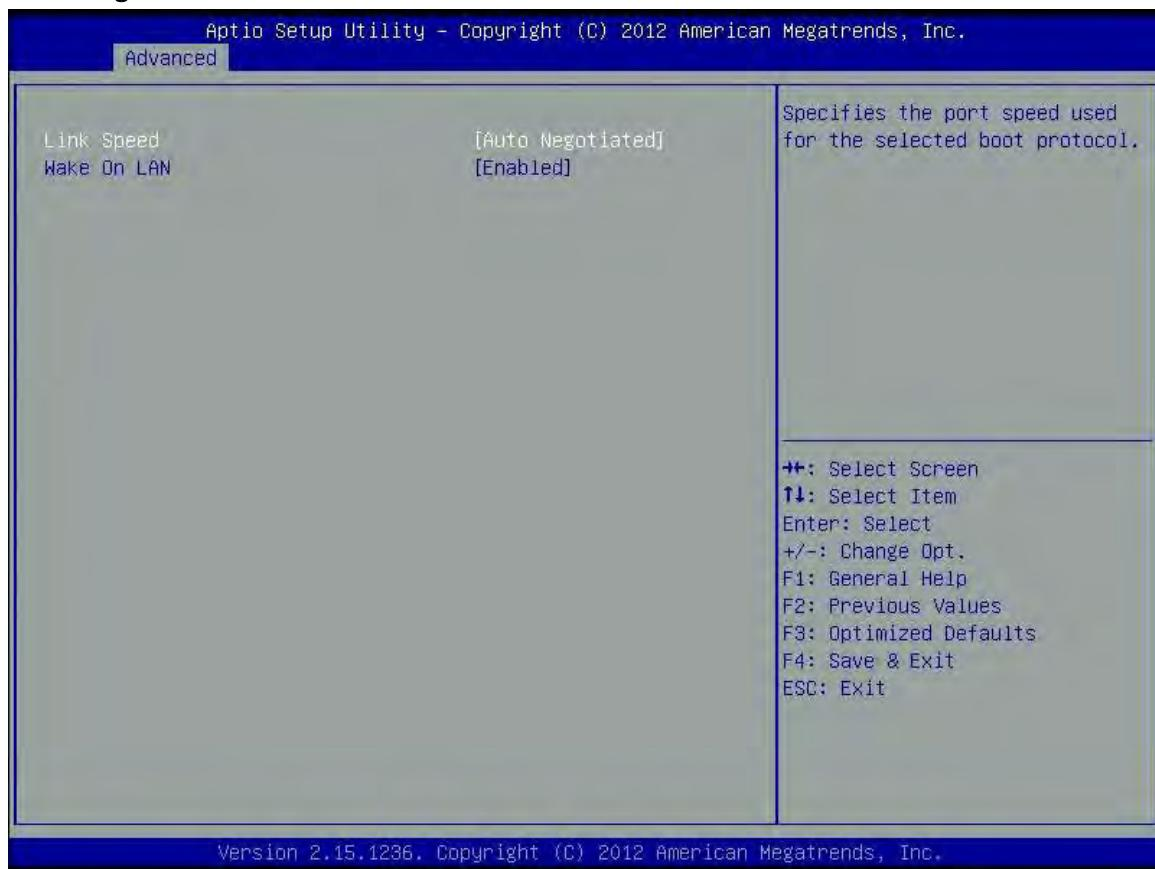
**Link Speed:** Specifies the port speed used for the selected boot protocol.
