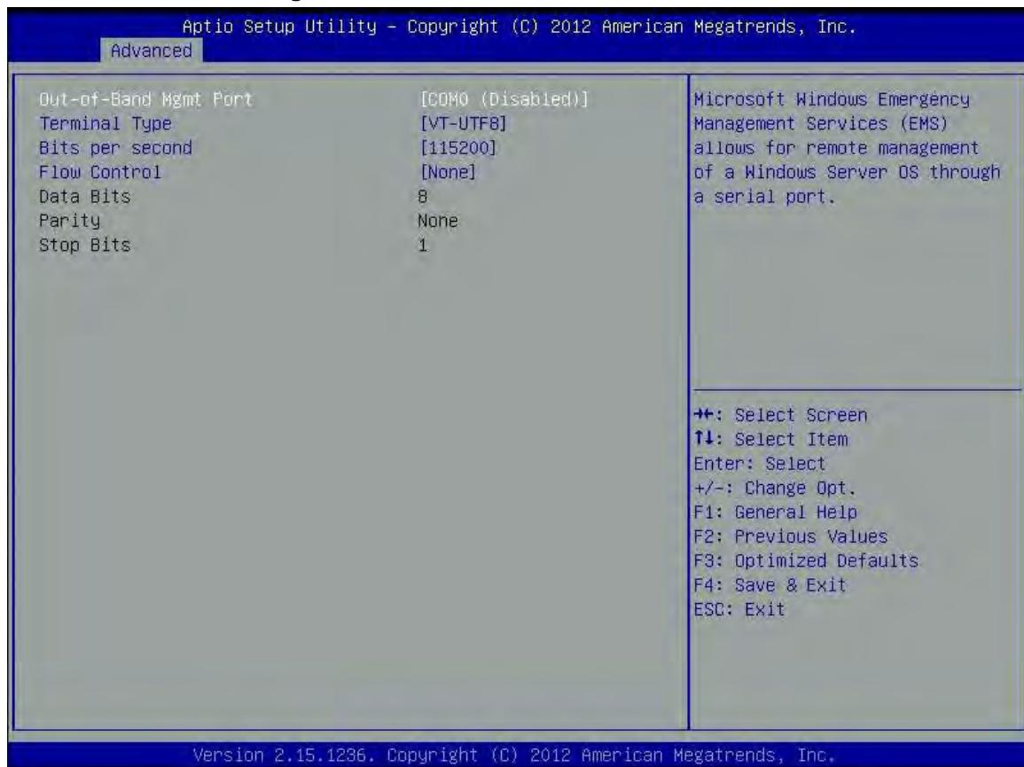
**Out-of-Band Mgmt Port:** Microsoft Windows Emergency Management Service (EMS) allows for remote management of a Windows Server OS through a serial port.
