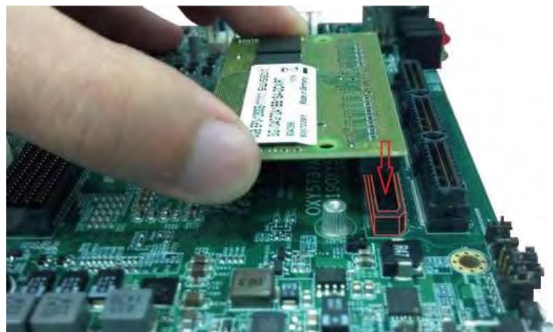
2. Align the memory module with the socket to make sure the notch aligns with the slot key on the socket.
