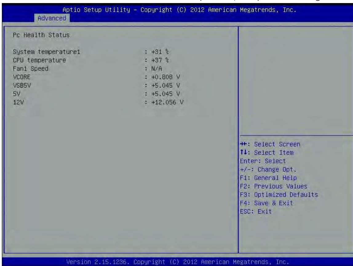
**System Temperature:** Detects and displays the current system temperature.
