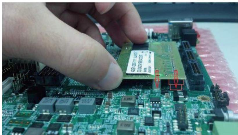
3. Insert the module firmly into the desired slot until the slot lock and secure the memory module.
