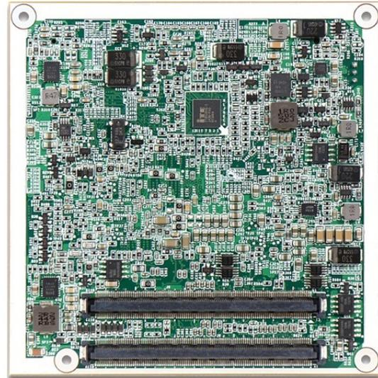
Portwell PCOM-B633VG is designed by Intel® 5<sup>th</sup> Generation Core™ i7/i5/i3 ultra low power processor with turbo-boost, SOL, IDER, iAMT 10.0 remote control which offer high speed and accurate responses suitable for medical healthcare systems and military seeker.
