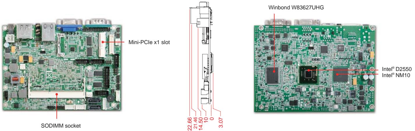
PEB-2772 takes advantage of the processor's performance and furthermore Portwell design the CPU/chipset on the backside of the board which is good for system thermal design. Customer could take this advantage to have an easy and perfect thermal solution which could solve the thermal of CPU.
