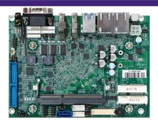
PEB-2773 build with Intel Atom™ processor E3900 series. Not only does it operates with TDP under 12W for fan-less applications, but it also supports industrial temperature range from -40°C to 85°C and wide voltage of power input from 12V to 24V.
