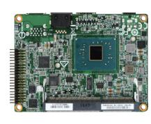
The PICO-6260 is a palm-sized fanless pico-ITX motherboard built with the latest 14 nm Intel® Apollo Lake Processor. Supports for two USB3.0 ports ensures fast data transmission with low-power con-sumption and support two com port to allow quick and lexible system expansions. Intel® I211AT Gigabit Ethernet controllers provide dual Gigabit Ethernet LAN access via the one RJ45 ports. PICO-6260 can design their own unique systems for Panel PC, Kiosk and Digital Signage applications.
