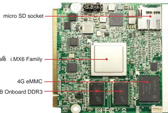
Qseven module based on Freescale™ i.MX6 family, ARM™ Cortex-A9, Solo / Dual / Quad core processor with onboard 1GB DDR3 (up to 2GB), PCIe 1-lane interface, VGA, HDMI, single LVDS 1-ch or dual LVDS (18/24-bit) 2-ch and CAN Bus.
