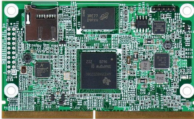
PSMRC-M310T is design as CPU module series with SMARC form factor. It is based on embedded TI™ AM3354 Single-core processor, an ARM® Cortex®-A8 processor. Best cost-effective entry model to replace original markets of ARM9 and ARM11.
