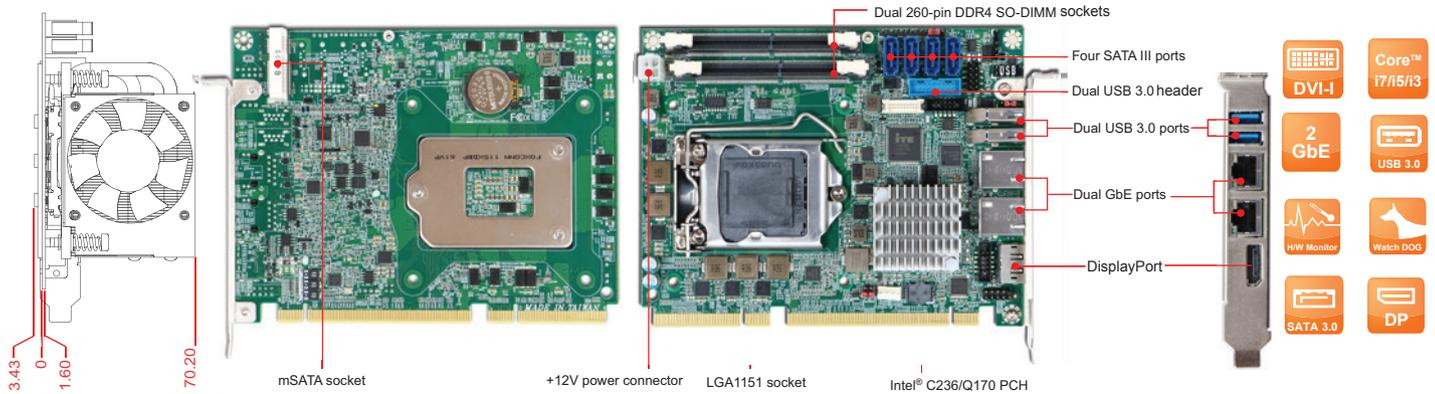
ROBO-6911VG2AR is based on Intel® C236/Q170 chipset to support both workstation and desktop processors. With flexible PCI Express configuration, ROBO-6911VG2AR is suitable for medical, industrial automation, and digital signage applications.
