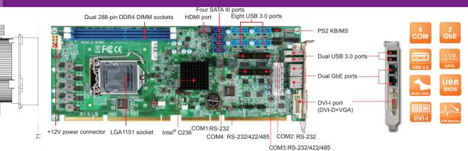
ROBO-8113VG2AR-KBL is based on Intel® workstation processors and C236 chipset. Built with fexible PCI Express configuration, ROBO-8113VG2AR-KBL is suitable for medical, industrial automation, and digital signage applications.
