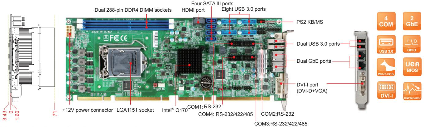
ROBO-8113VG2AR-Q170-KBL, based on Intel® desktop processors and Q170 chipset, and built with flexible PCI Express configuration, is suitable for medical, industrial automation and digital signage applications.
