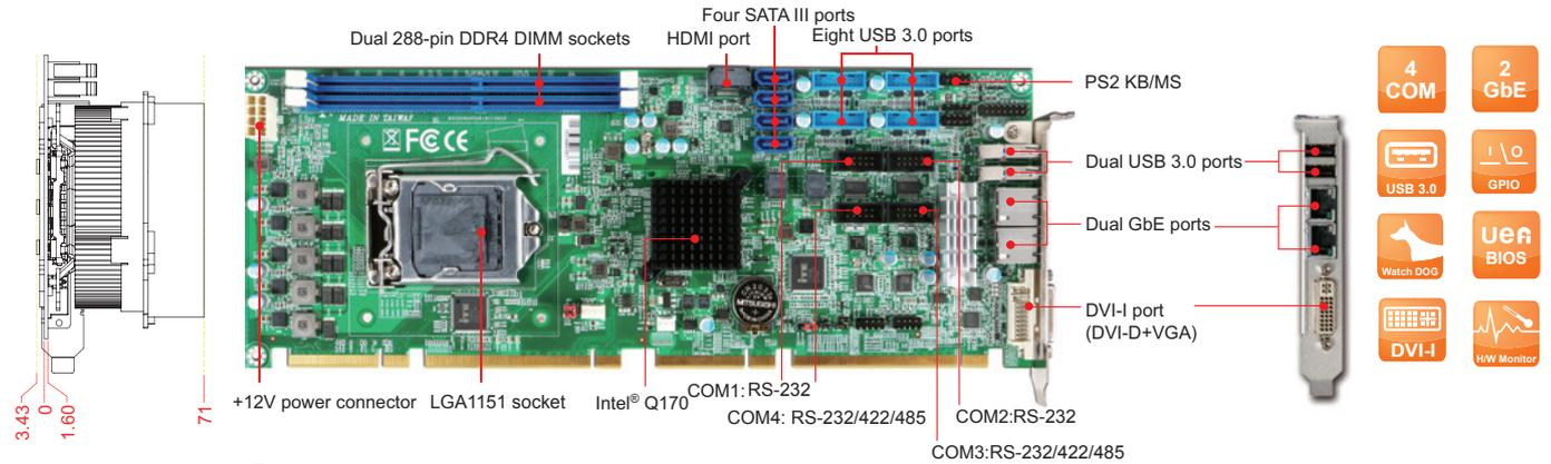
ROBO-8113VG2AR-Q170 is based on Intel® desktop processors and Q170 chipset. Built with flexible PCI Express configuration, ROBO-8113VG2AR-Q170 is suitable for medical, industrial automation, and digital signage applications.
