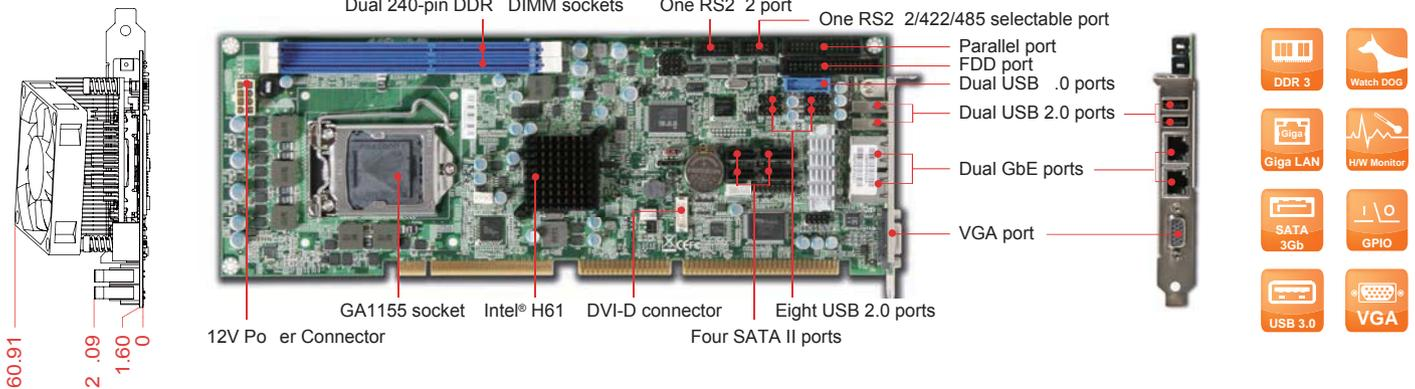
ROBO-8780VG2A is based on Intel® H61 chipset and Intel® Core™ i3/i5/i7 processors. It supports VGA and on board DVI-D display. It's suitable for Medical, Industrial automation, and digital signage applications.
