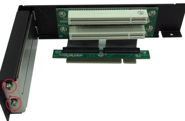
3. Insert PCI add-on card into PCI slot from riser card.
