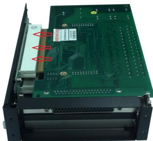
4. Insert add-on card screw to firmed the add-on card, and insert the PCI riser's bridge board to motherboard PCI slot.
