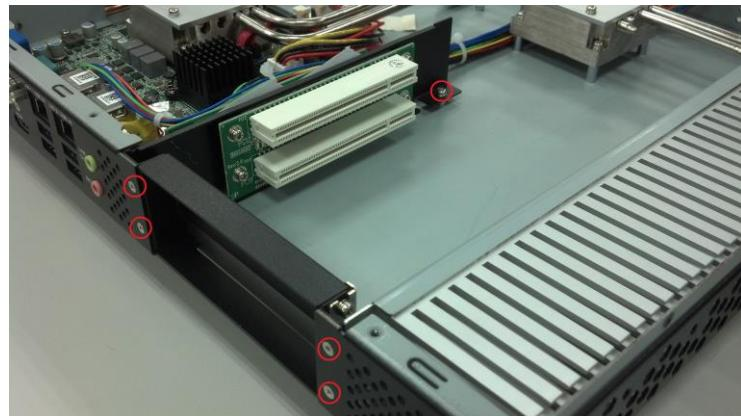
2. Remove the screws to set PCI add-on card on PCI riser card.
