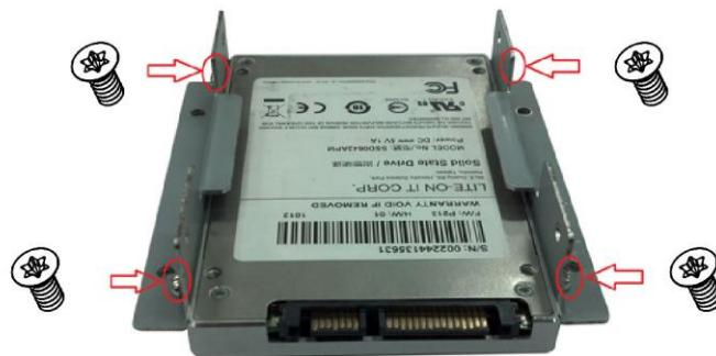
4. Insert each of left and right side screws, to set 2.5" HDD into system.
