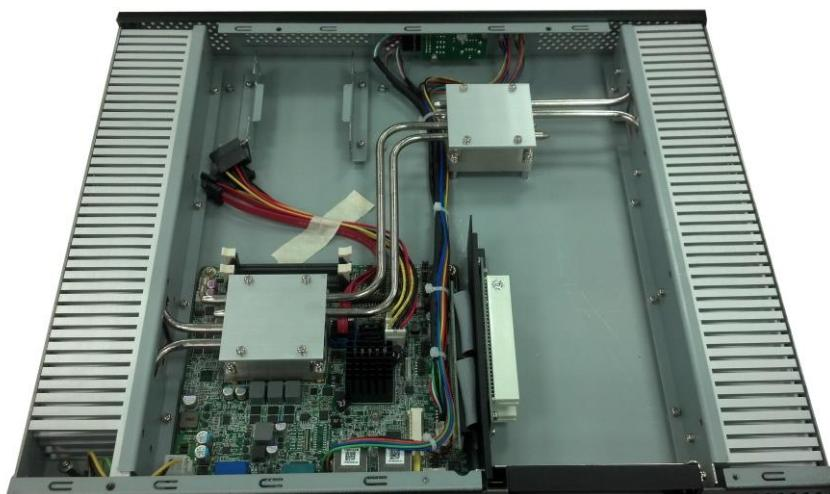
2. Remove 4 screws from the screw hole to take off the HDD bracket.
