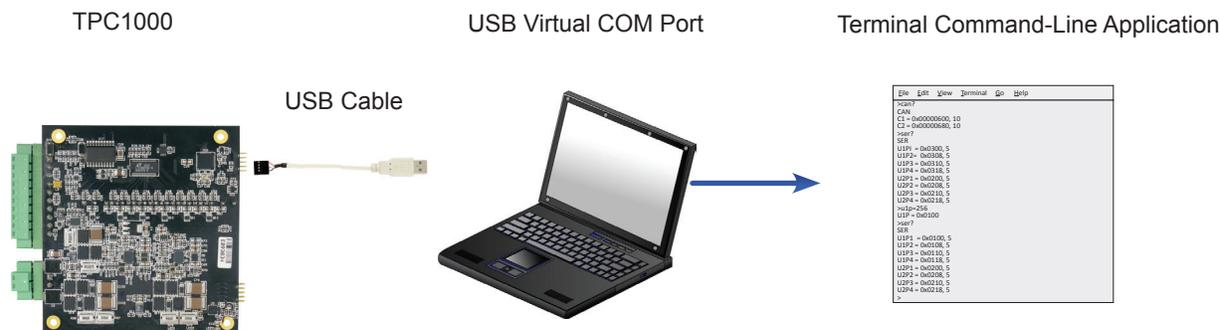
**Figure 10: TPC1000 accessed via an asynchronous serial port**
