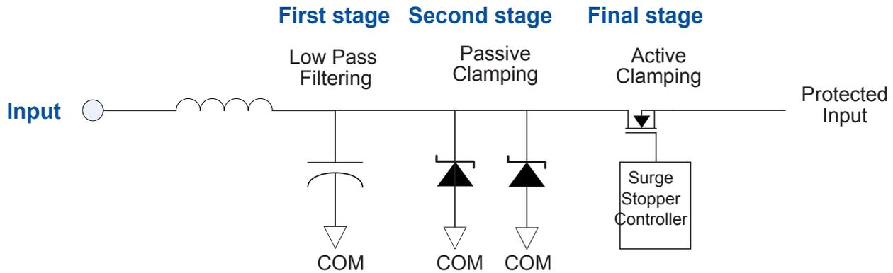
The first stage is a waveform modification that employs a low pass filter to eliminate unwanted high frequencies from entering the system.
