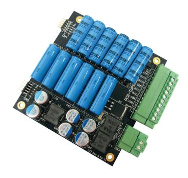
The TUP1000 is a Small Form Factor (SFF)1 DC-DC converter using ultra capacitors versus batteries to provide seamless UPS backup capabilities. This high performance power supply can produce 35 watts @ +5VDC or 42 Watts @ +12VDC.
