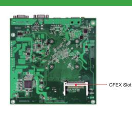
WADE-8078 is the first Portwell off-the-shelf Mini-ITX embedded board product based on the Intel® Atom™ processor E3800 product family with memory and PCI Express controller integrated to support one-channel DDR3L memory and PCI Express 2.0 lanes.Portwell has taken advantage of such technology to furnish a series of products that meets multiple industrial requirements for cost effectiveness, reliable performance and a high level of data integrity and uptime.
