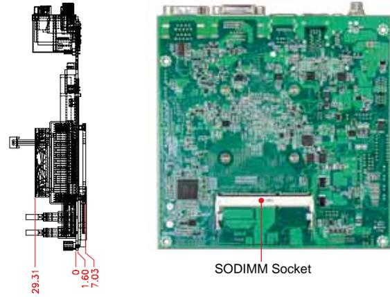
WADE-8079 is based on Intel® Atom™ processor E3800 product family with memory and PCI Express controller integrated to support two-channel DDR3L memory and PCI Express 2.0 lanes. Portwell has taken advantage of such technology to furnish a series of products that meets multiple industrial requirements for cost effectiveness, reliable performance and a high level of data integrity and uptime.
