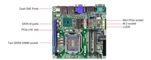
WADE-8211 is based on Intel® Q370 chipset and Desktop processors including Intel® 8th Gen Core™ i3/i5/i7 SKU. This board supports DDR4 ,PCIe 3.0, and SATAIII. Those fratures help you to build high performance and stabile system.
